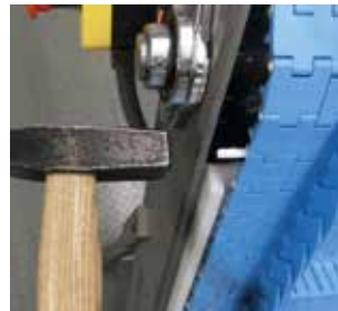
3 Gently tap its head into retaining position
